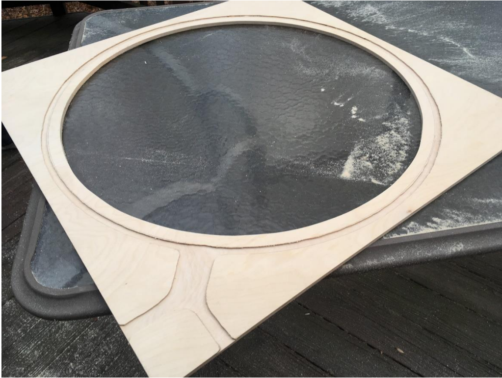
Figure 6 Underside of Roadbed After Cutting and Routing
