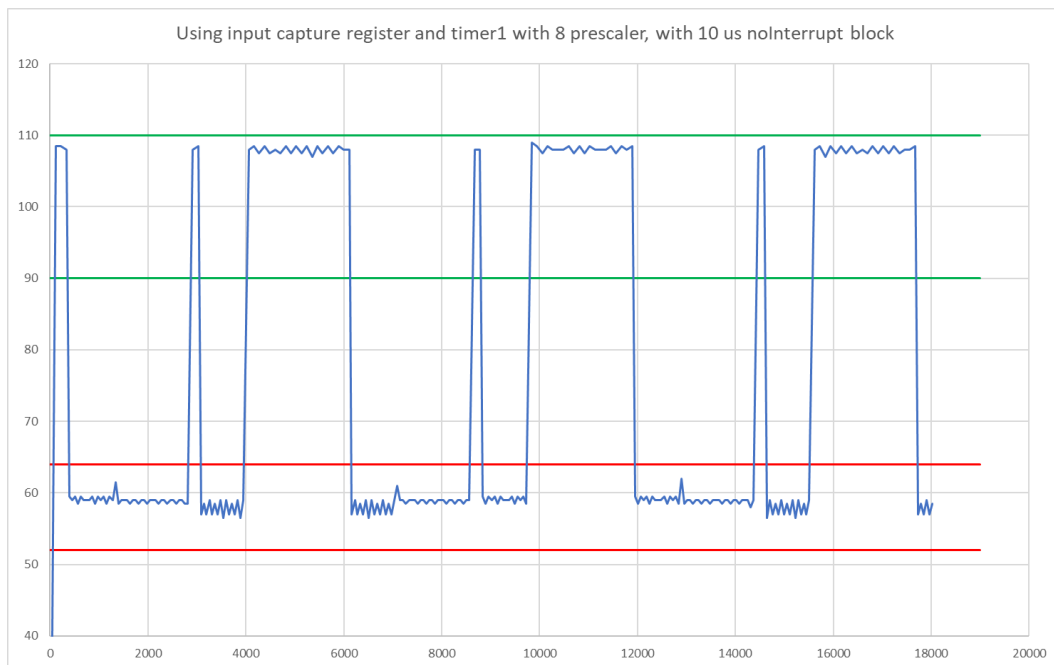
Figure 12 Input Capture Register with 10\mu\text{s} noInterrupts Block
